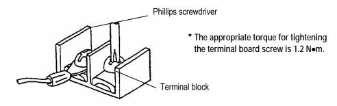
Figure 5.10 Connecting a Cable to Terminal Block
